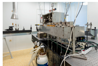
Vacuum manifold for absorption reference cells development and filling.
