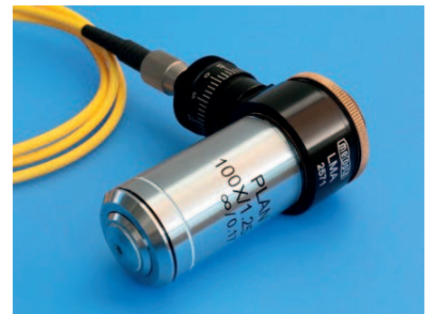
Compact device for creating optical tweezers attachable to a Raman microscope.
