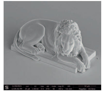
Structure of lion prepared by two photon lithography system. With permission of IQSnano.
