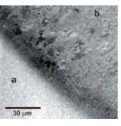
Ultrafine grained copper sheet as inserted in the ultrahigh vacuum (a) and after ion beam cleaning that reveals the crystalline structure (b). Landing energy of electrons: 2 keV.
