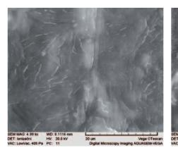
Inner surface of vascular catheters in ESEM.
