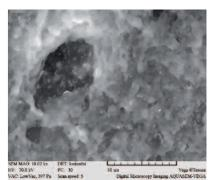
Sealing ring surface corroded in HNO<sub>3</sub>.
