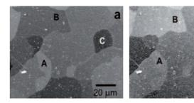
The X210Cr12 steel heated to the semi-solid state at 1265°C, deformed 2:1 at 800°C and cooled down; observation under UHV conditions: standard image with backscattered electrons (BSE) at 6 keV (a), full BSE image at 500 eV (b) and at 50 eV (c); boundary between areas in-situ cleaned with ions and the as-inserted state (d); sample annealed at 500°C for 60 min.: standard BSE image at 8 keV (e) and full BSE image at 500 eV (f).
