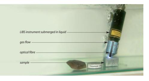
LIBS excels in instances where on-site, real-time, and on-line measurements in various production phases are required (e.g. for metal identification problems). Different types of steel (e.g. FV520, NAG, 17/4, and 18/13) can be identified simply by following some of the representative elements (e.g. Mo, Ni, and Ti).
