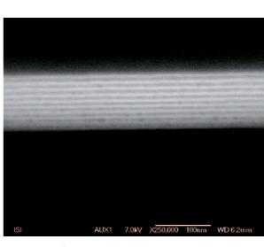
Cross-section of a Mo-Si multilayered nanostructure.
