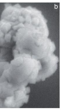
Spinel crystals growing on the ceramic surface in the aluminum alloy based metal matrix composite: (a) 1 keV image with the complete emission of backscattered electrons acquired, (b) standard micrograph at 10 keV.
