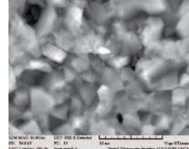
Uncorroded surface of the alumina ceramic.
