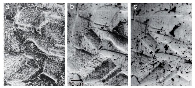
Surface of the polycrystallinic copper sheet imaged at electron energies 5 keV (a), 200 eV (b) and 10 eV (c).
