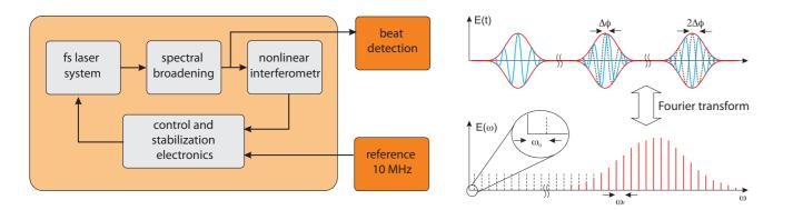
Block diagram of the optical synthesizer (left) and time and spectral expression of the pulsed light output, the optical comb (right).
