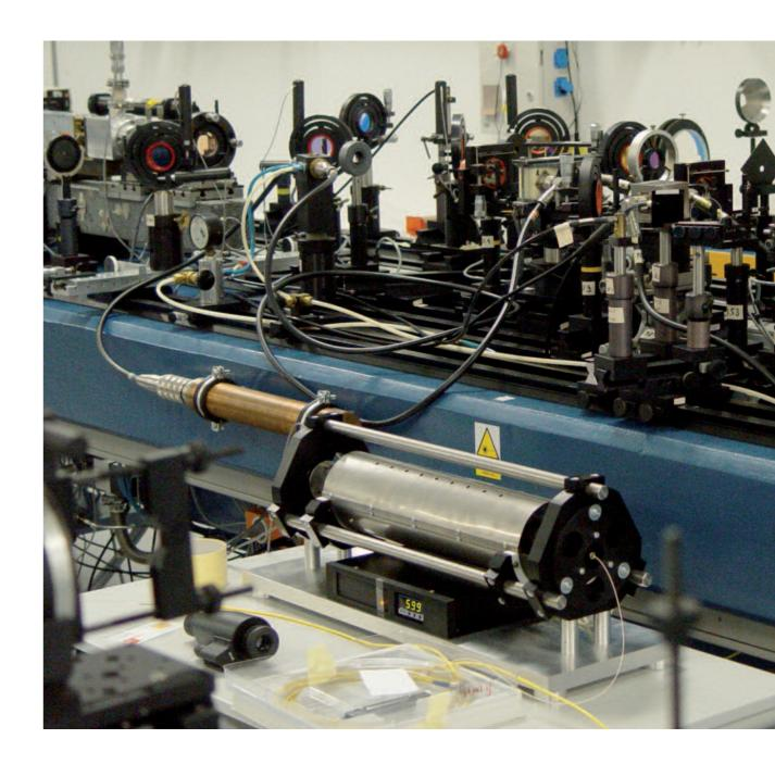
Detection and control is fully automatic and the instrument is controlled by several signal processors. The laser operates at the 1315 nm wavelength, in the telecommunication spectral range. It can also serve as an etalon for optical telecommunications.
