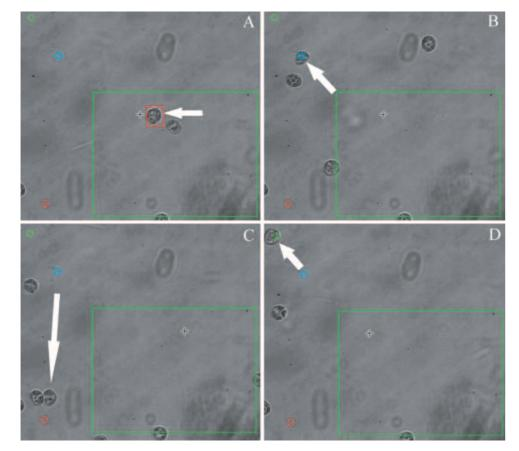
Example of 3D manipulation inside transparent (living) objects. A small crystallite is optically trapped inside living Amoeba. Despite movement of the whole sample and cytoplasmic streaming, the crystallite is spatially fixed.
