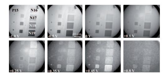
Atomically flat twodimensional crystals of lead on the silicon surface, imaged by means of the dark-field diffraction contrast.
