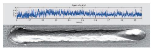
A record of plasma radiation intensity during laser welding.
