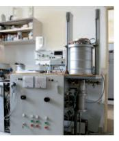
Vacuum furnace of our own design and manufacture suitable for vacuum brazing and annealing of small-sized components:
