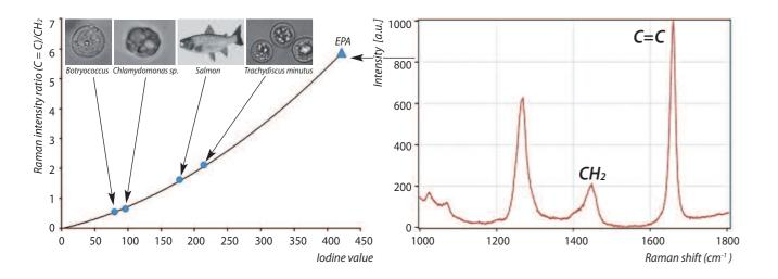
The degree of unsaturation of the constituent fatty acids can be quantified by the iodine value frequently used in food and chemical industry. lodine value can be estimated using the calibration curve employing the ratio of the characteristic peaks in the Raman spectra (here for the three algal and one fish species). It can be seen that the highest iodine value is for Eicosapentaenoic acid (EPA) which belongs to the family of omega-3 fatty acids.
