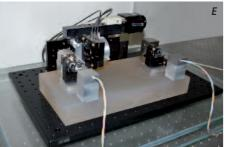
System for measuring of the refractive index of air with He-Ne lasers (left, figure C).
