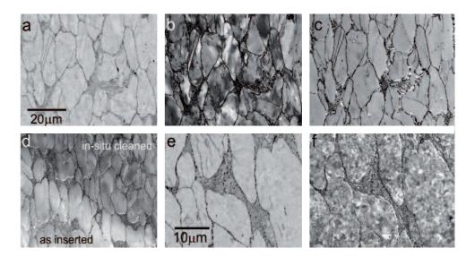
When reducing the landing energy of electrons below some 30 eV, their reflectance becomes inversely proportional to the local density of electronic states, which is characteristic for the crystalline system and its spatial orientation. Thus, the energy dependence of the reflectance can serve to fingerprinting orientation of a crystalline grain.
