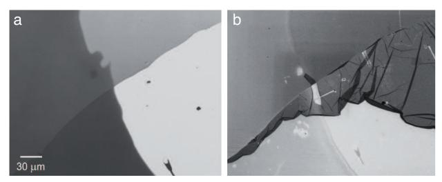
A patterned multilayer structure imaged under different surface sensitivities controlled with energy of electrons; image at 9800 eV (a) and 850 eV (b).
