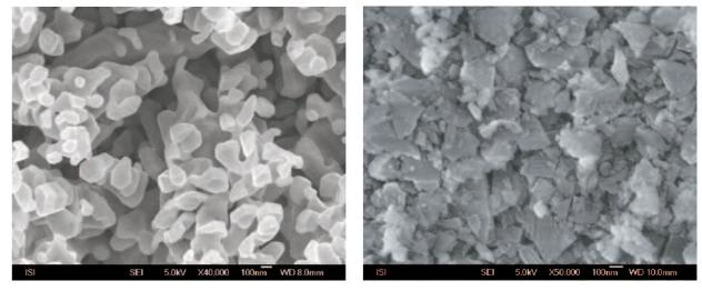
Iron oxide deposited on the silicon surface.
