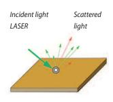
Diagram of principles behind Raman spectroscopy: Scattered light of the same wavelength as incoming laser *Raman shift from the* incident laser energy gives a Raman spectrum. Different materials have characteristic Raman spectra.
