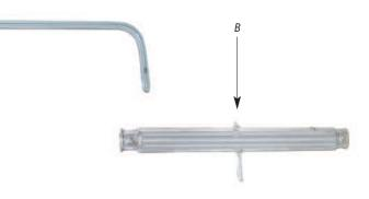
lodine cell with Brewster angle windows designed for a He-Ne laser etalon of optical frequency at 633 nm wavelength (A) and iodine cell with wedged windows (B).
