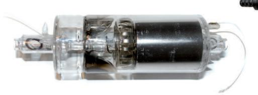
**ECL lasers for measurement and spectroscopy.** Traditional He-Ne lasers operating in the visible spectral range are only tunable within a very narrow range. Laser diodes perform much broader tuning range but do not operate in a single-frequency regime and are thus not suitable for demanding applications like interferometry and spectroscopy - for example, for gas analysis. We designed semiconductor laser technology with an extended cavity, which
