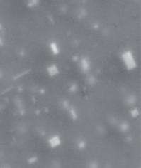
Precipitates in the Al-Mg-Si alloy shown at optimized energy of electrons (a) in comparison with the conventional image (b).
