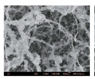
Carbon based nanostructure with iron particles on a silicon substrate.
