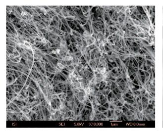
Structure of randomly grown carbon nanotubes.
