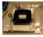
Example of the multiaxis interferometer for the 3D positioning of the sample for AFM microscopy.
