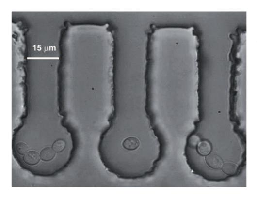
Example of the microfluidic structure of cultivation microchambres with living yeast cells. The side chambers are occupied by non-stressed cells that divide, and a non-dividing stressed cell is placed in the middle chamber. The cells were positioned in the chambers by the optical tweezers.
