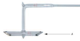
Cells filled with superpure gasses (acetylene <sup>13</sup>C<sub>2</sub>H<sub>2</sub>, Methane, Xenon, Krypton) or saturated vapor of lodine, Cesium, Rubidium, etc. Cells filled with iodine serve as s reference for the primary etalons of (wave)length. The frequency shifts of iodine cells made at ISI are the smallest in the world (below 1 kHz of the optical frequency). The technology of the ISI allows the preparation of cells filled with various media based on application requirements.
