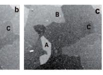
Polycrystalline aluminium in-situ cleaned and annealed, UHV imaging with full BSE emission at 7.8 eV (a), 17.4 eV (b), and 24.6 eV (c); orientation of the labelled grains: A ~(101), B ~ (111), C~(001).
