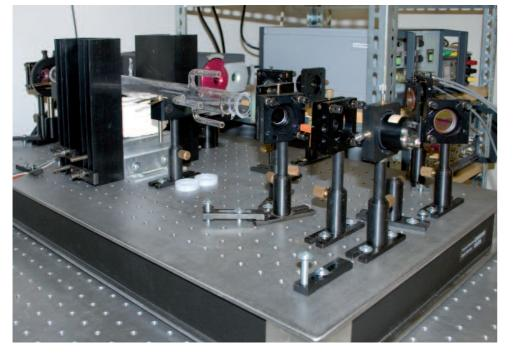
Stabilized system at the 1315 nm wavelength. This system was designed according to the specifications and needs of the "Prague Asterix Laser System" (PALS) research center. We designed a system based on a narrow-linewidth DBR laser diode operating as a "master oscillator" at the front end of a cascade of optical amplifiers. This is a laser with fiber optic output with a frequency stabilized through linear absorption in vapor of dissociated lodine.
