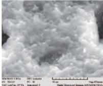
Uncorroded surface of an O-ring sealing.
