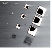
Areas imaged at 1000 eV with the contrast proportional to the dopant density and at 3 eV with the dynamic contrast enablina critical dimensions to be measured.
