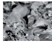
Internal strain inside grains in hot rolled ferritic steel.
