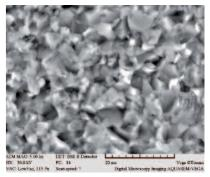
Ceramic surface corroded in H<sub>3</sub>PO<sub>4</sub>.
