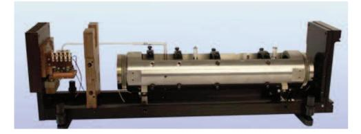
including computer control. Relative stability of the laser is on the 10<sup>-11</sup> level for 1s integration time. It is used for the calibration of He-Ne laser sources for interferometric systems.
