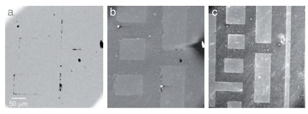
P-type doped patterns on the n-type silicon substrate imaged by means of conventional detectors (a, b) and using the cathode lens mode (c).
