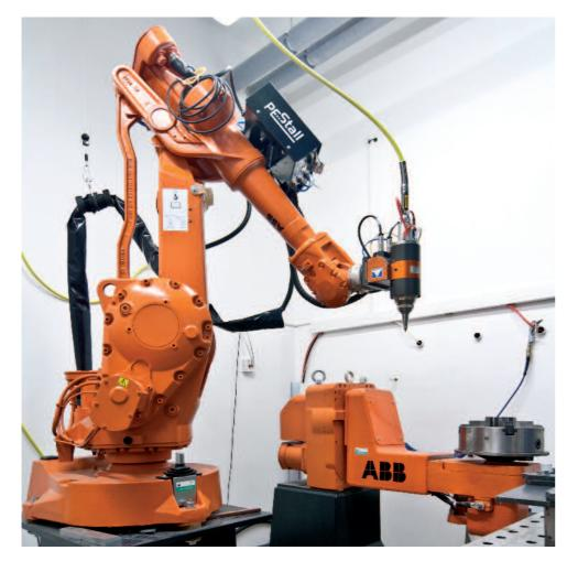
Example of laser-hardening shaft
