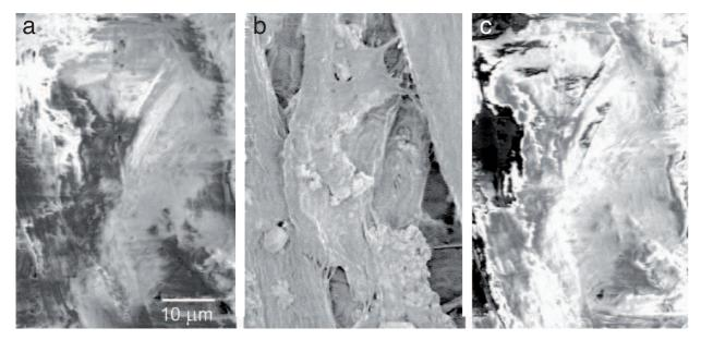
Surface of writing paper in its original nonconductive status, imaged below (a), at (b) and above(c) the optimum electron energy for suppressed charging.
