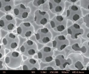
Nanostructured golden electrodes of electrochemical sensors.
