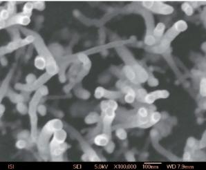
Magnified structure of the carbon nanotubes.
