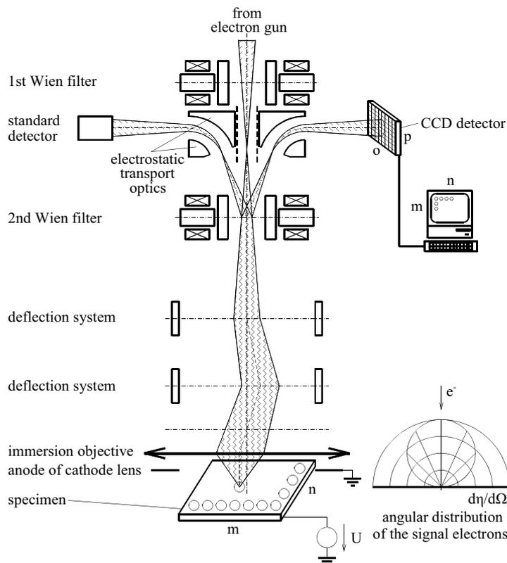
Figure 1: VLESEM with EBCCD detector.
